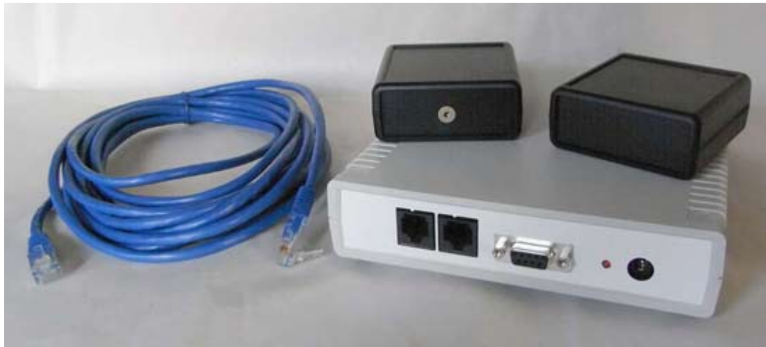
The component parts of LaserMaze – Interface, Laser and Sensor modules, and RJ45 cabling
